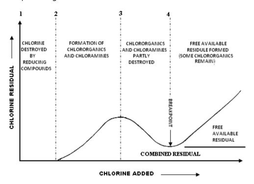
Between points 2 and 3, the chlorine reacts with organics and ammonia naturally found in the water. Some combined chlorine residual is formed – chloramines.
